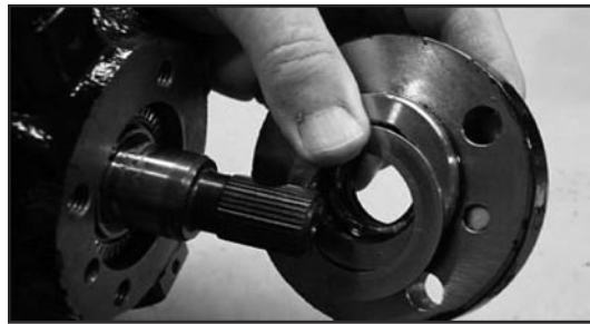
Figure 10. Reinstalling Thrust Washer.
